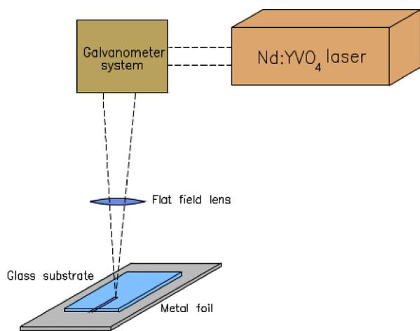
**Fig 3.** Experimental setup for the laser backwriting technique. The laser was combined with a galvanometer system formed by mirrors that addresses the laser beam, so no need of sample movement was needed. A flat field lens with 100 mm focal length was employed in order to focus the laser over the substrate and provided a working area of 80x80 mm<sup>2</sup>.
